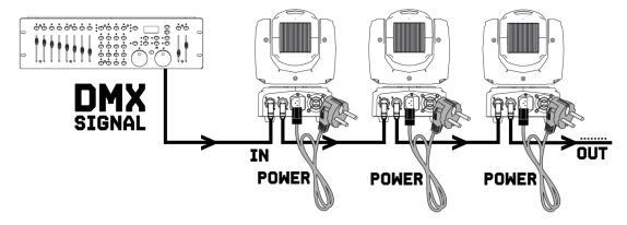
**CAUTION!** At the last unit, you must close the DMX line with a terminating resistor. Take an XLR connector and solder a 120 0hm resistor between signal (+) and signal (+) and connect it to the DMX output of the last unit in the line.
